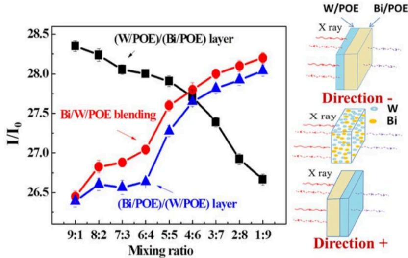
Figure 23: Dose ratio of X-ray passed through the blending and layered composites, with different layer thickness ratios. [10]
