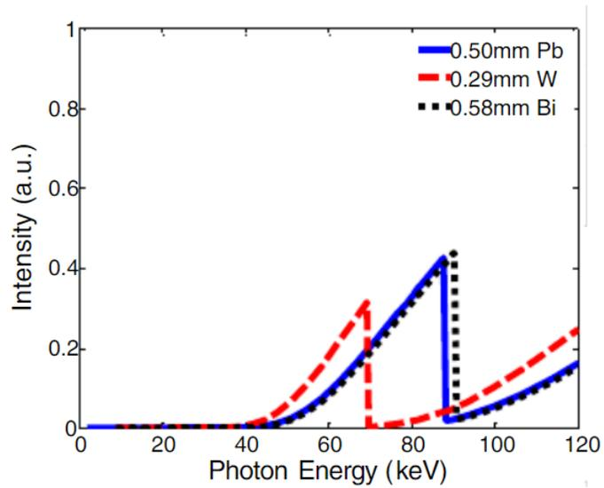
Figure 20: Transmission spectra of W, Bi, and 0.50mm Pb at the same weight. [10]
