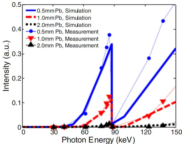
Figure 18: X-ray transmission intensity between simulated and measurement results across 0-150keV energy transmissions. Three Pb sheets with varying thicknesses are studied. [10]
