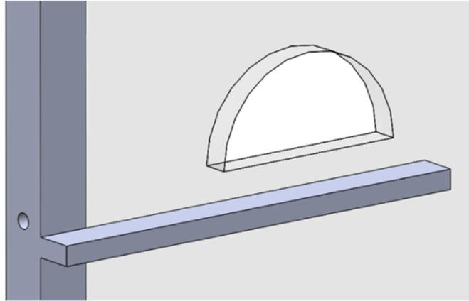
*Figure 12: Image showing the ledge attached to the outer frame that supports the hand plate*
