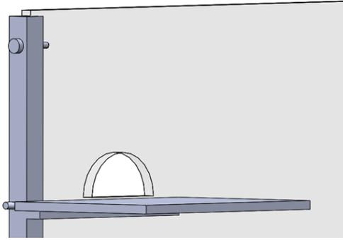
*Figure 16: The image shows the hand plate in the final position, where it is ready to use.*
