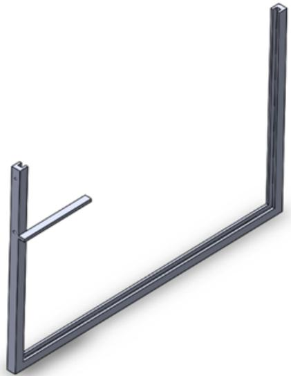
*Figure 10: Image shows the outer frame with slots*
