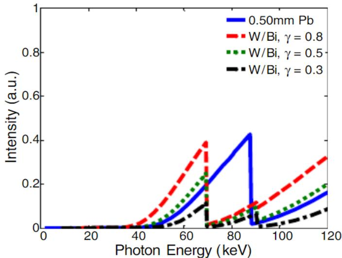
The double-layer W/Bi sheet is observed in different thickness ratios at  $\gamma = 0.8, 0.5,$  and  $0.3$ . The thickness of W is fixed at 0.20 mm. The thicknesses of Bi are 0.05 mm, 0.20 mm, and 0.47 mm for the thickness ratio of 0.8, 0.5, and 0.3, respectively.
