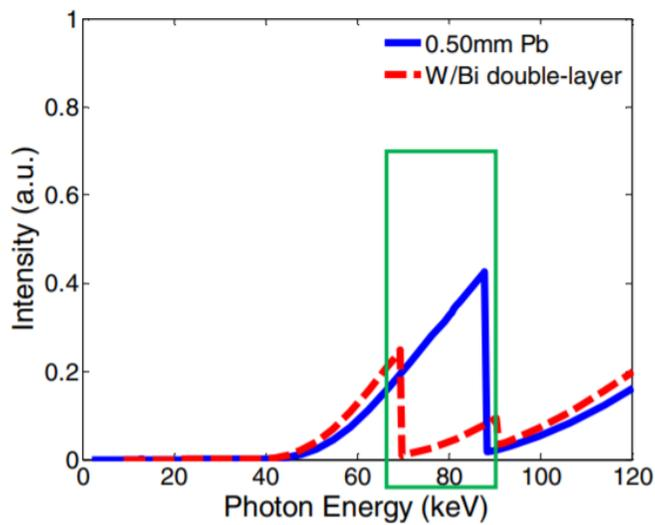
Figure 21: Transmission spectra versus energy of 0.5mm Pb sheet and double-layer W/Bi sheet at same weight, with W and Bi thickness of 0.29mm and 0.58mm respectively. [10]
