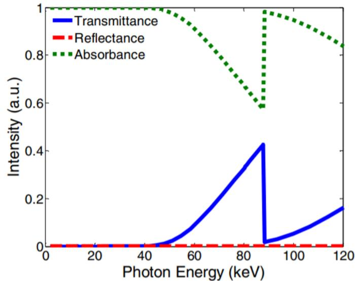
Figure 19: Transmission, reflection and absorption spectra versus energy of a 0.5mm Pb sheet. [10]
